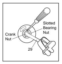
driver in one of the slots in the slotted bearing nut. Lightly tap the screwdriver with a hammer to turn the slotted bearing nut counterclockwise until the arms are no longer loose. **Do not overtighten the slotted bearing nut.** When the slotted bearing nut is properly tightened, tighten the crank nut.
